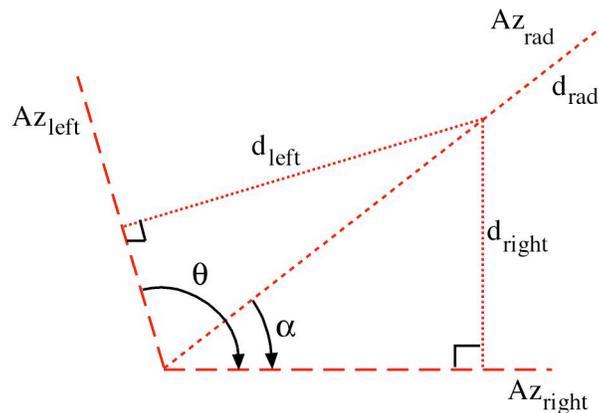
The angle  $\theta$  is the difference between the two known azimuths,  $Az_{left}$  and  $Az_{right}$ . The offset from the right traverse line to the object is  $d_{right}$ , while the offset from the left traverse line to the object is  $d_{left}$ . Because the offsets are measured at right angles to the traverse lines, their azimuths are also known.
